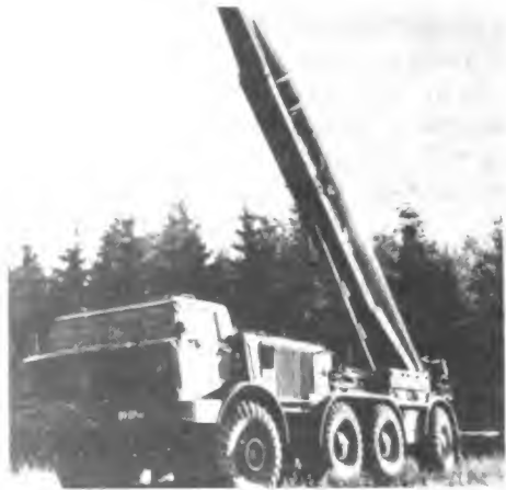
Figure 6-22. Free Rocket Over Ground (FROG). FROG battalions give nuclear/chemical striking power to tank and motorized rifle divisions. The older FROG-3 (left) is carried on a tracked launcher, while the newest model, the FROG-7 (right), is transported on a single-rail launcher mounted on a ZIL-135 truck.
